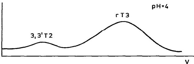
Fig. 1. Elution pattern obtained when the reaction mixture from the chloramine-T labelling of rT3 was chromatographed. Eluent, 30% ethanol; pH = 4.
